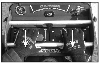
Grab the rear handle bar with your thumbs and the steering control handles with your fingers. Pull the steering control handles back, towards you, at the same time. Pull back slightly to move slowly in reverse. Pull back harder to increase the speed of your reverse movement.
